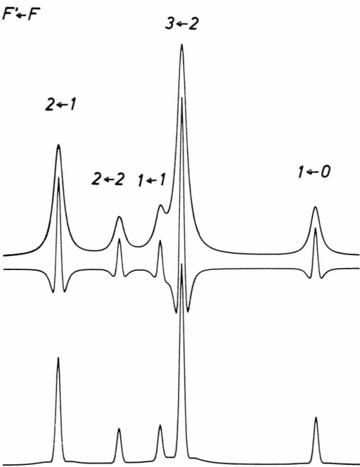
Fig. 3. Simulation of the 110-211 hfs-pattern of CD 2 FCN assuming Lorentzian line profiles with 150 kHz full width at half height (upper trace), -f(\Delta n)^2(y(n+1) - 2 \cdot y(n) + y(n-1)) with f = 0.7 and (\Delta n) the half halfwidth in units of frequency steps (here 10 kHz/step) (centre trace), and the sum of the two traces (lower trace).
